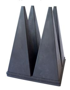
The 3630 series Wide-band hybrid pyramid EM absorber is an 80 mm high absorber that measures 200 mm x 200 mm. It shows good absorption performance in the wide band between 30 MHz and 18 GHz when combined with 6.3 mm thick Ferrite absorber tiles (Part nr. 3600-63). The hybrid pyramid absorber is made out of a carbon-loaded polystyrene and is tuned for perfect performance over Ferrite absorber tiles.
