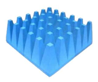
The 3660 series PU foam based Hybrid absorbers product is similar to our standard pyramid absorbers, but having the tips of the pyramids truncated. This saves space in small chambers and provides a more rugged product, eliminating the possibility of tip breakage.
