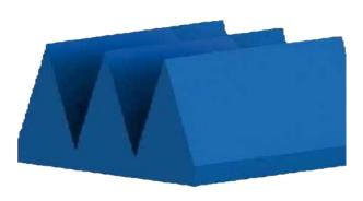
PU foam based wedge absorbers has the properties similar to the pyramid absorbers with same height, it also has excellent performance in 100MHz-110GHz. It is mainly applied in large compact anechoic chamber and tapered anechoic chambers, the main advantage is to reduce the back scattering of pyramid absorbers and obtain higher quietness of quiet zone.
